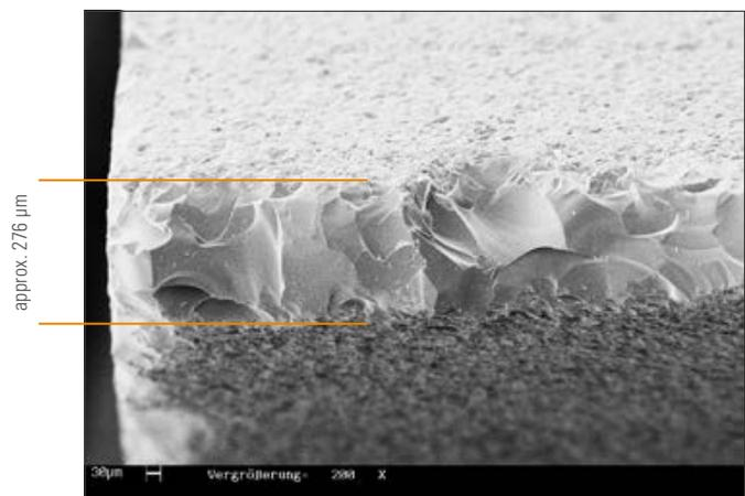
Lithium disilicate ceramic, SEM picture, 200 x
